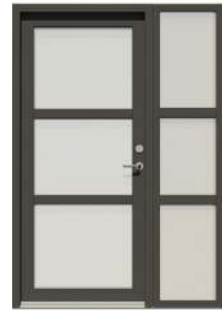
8. Glazed entrance door with integrated side light
